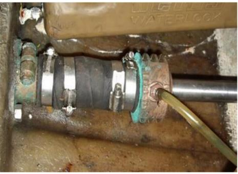
Subsequently, I have found that once at rest the stern glands are doing their job because they eventually seal out the ingress of seawater when the shafts are not revolving.
